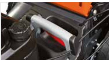
Practical, lever-operated cutting height adjustment system.
