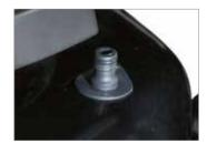
The quick-fit "Deck Wash System" connector on the mowing deck makes it possible to direct water inside the deck for quick and easy cleaning of the cutting mechanism (103, 123).
