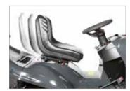
Comfortable operating position thanks to a seat that can be adjusted directly by the seated driver (123/22 V).
