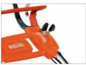
Model **VBD** is equipped with stepless traction control so that ground speed can be adapted continuously to match the needs of the job.
