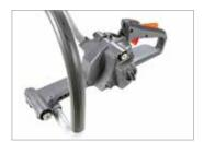
Anti-vibration system composed of 6 vibration dampers - 2 spring dampers and 4 rubber stops: interposed between the handle and the crankcase, the dampers ensure optimal isolation from vibration for enhanced operator comfort.
