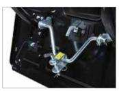
The towing hitch, fitted as standard, makes the machine even more versatile, allowing it to tow a trailer or lawn roller (103, 123).
