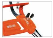
Model **VK** is equipped with stepless traction control so that ground speed can be adapted continuously to match the needs of the job.
