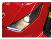
Halogen headlights and LED worklights ensure a good view of the cutting area, even in low light conditions.
