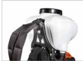
Fastening the shoulder straps directly to the tank on model MB 90/MB 900 has made it possible to lower the mistblower's centre of mass to minimise oscillation during movements.
