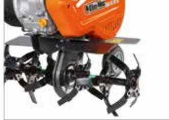
46cm rotor with three elements on each side, reducible to 32-22 cm.
