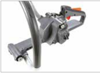
Anti-vibration system composed of 6 vibration dampers - 2 spring dampers and 4 rubber stops: interposed between the handle and the crankcase, the dampers ensure optimal isolation from vibration for enhanced operator comfort.
