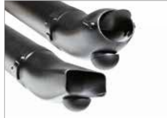
Two air delivery nozzles supplied as standard: rectangular/round section, both equipped with hemispherical support so the tube can rest on the ground on level terrain to reduce operator fatigue (BV 901).
